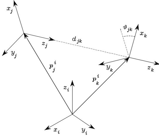
**Fig. 2.19.** Coordinate transformation at the cut joint
