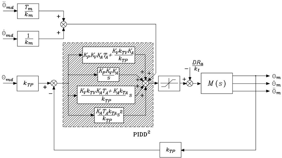
Fig. 8.17. Equivalent control scheme of PIDD<sup>2</sup> type
