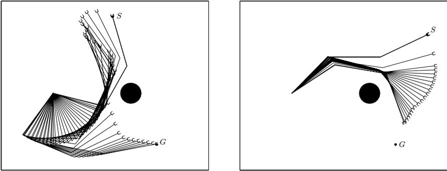
**Fig. 12.16.** Examples of motion planning via artificial potentials acting on control points for a planar 3R manipulator; *left*: planning is successful and leads to a collision-free motion between the start  $S$  and the goal  $G$ , *right*: a failure is reported because the manipulator is stuck at a force equilibrium
