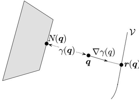
**Fig. 12.6.** The retraction procedure for connecting a generic configuration  $\mathbf{q}$  in  $\mathcal{C}_{\text{free}}$  to  $\mathcal{V}(\mathcal{C}_{\text{free}})$
