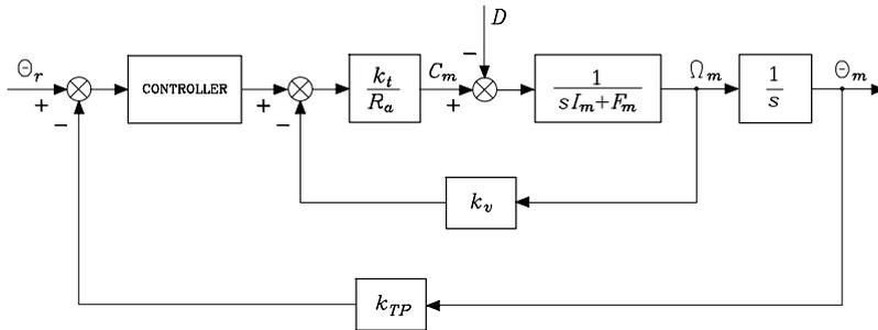
Fig. 5.9. General block scheme of electric drive control
