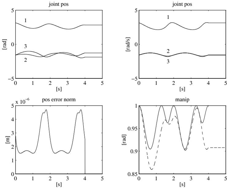
**Fig. 3.19.** Time history of the joint positions, the norm of end-effector position error, and the manipulability measure with the Jacobian pseudo-inverse algorithm and manipulability constraint; *upper left*: with the unconstrained solution, *upper right*: with the constrained solution
