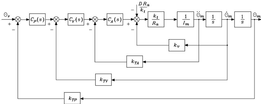
Fig. 8.6. Block scheme of general independent joint control
