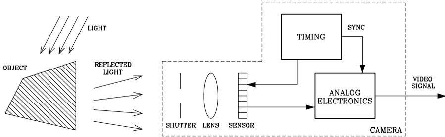
Fig. 5.22. Schematic representation of a vision system
