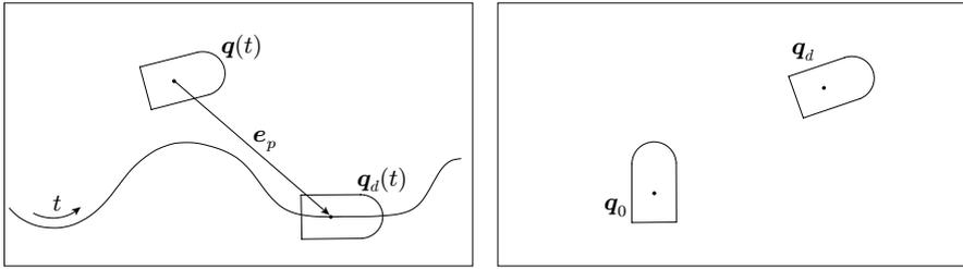
**Fig. 11.13.** Control problems for a unicycle; *left*: trajectory tracking, *right*: posture regulation
