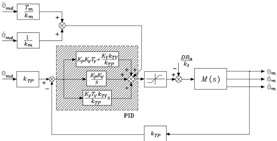
Fig. 8.16. Equivalent control scheme of PID type
