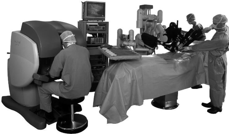
**Fig. 1.40.** The da Vinci robotic system for laparoscopic surgery (courtesy of Intuitive Surgical Inc)
