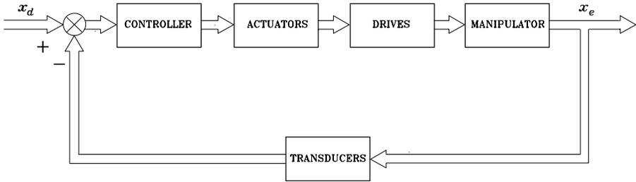
**Fig. 8.2.** General scheme of operational space control
