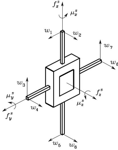
Fig. 5.17. Schematic representation of a Maltese-cross force sensor
