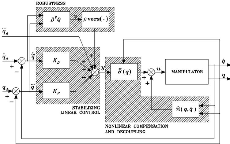
Fig. 8.23. Block scheme of joint space robust control
