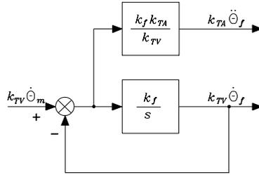
Fig. 8.11. Block scheme of a first-order filter
