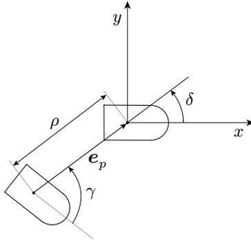
**Fig. 11.18.** Definition of polar coordinates for the unicycle
