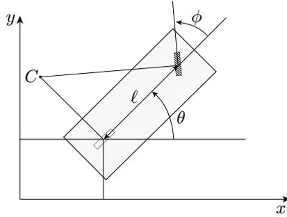
**Fig. 11.4.** Generalized coordinates and instantaneous centre of rotation for a bicycle
