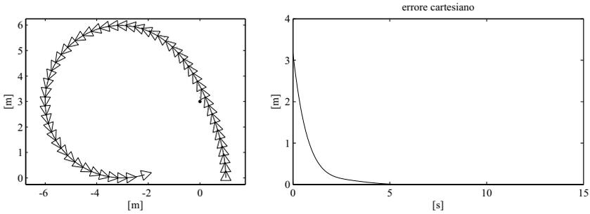
**Fig. 11.14.** Tracking a circular reference trajectory (*dotted*) with the controller based on approximate linearization; *left*: Cartesian motion of the unicycle, *right*: time evolution of the norm of the Cartesian error  $e_p$
