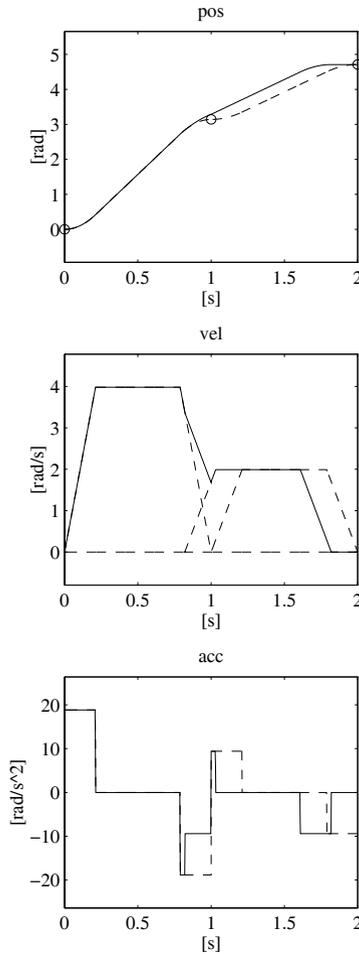
**Fig. 4.10.** Time history of position, velocity and acceleration with a timing law of interpolating linear polynomials with parabolic blends obtained by anticipating the generation of the second segment of trajectory
