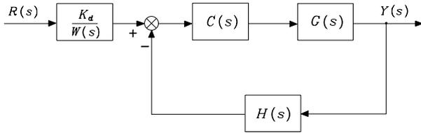
**Fig. C.3.** Feedback control structure with inverse model technique
