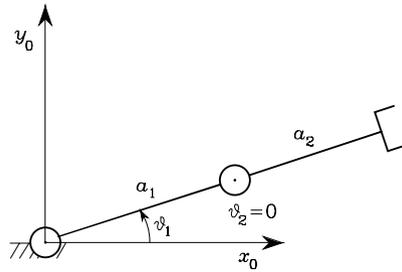
**Fig. 3.3.** Two-link planar arm at a boundary singularity
