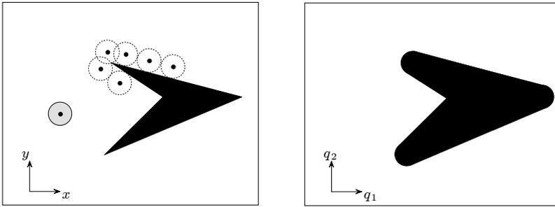
**Fig. 12.2.**  $\mathcal{C}$ -obstacles for a circular robot in  $\mathbb{R}^2$ ; *left*: the robot  $\mathcal{B}$ , an obstacle  $\mathcal{O}_i$  and the growing procedure for building  $\mathcal{C}$ -obstacles, *right*: the configuration space  $\mathcal{C}$  and the  $\mathcal{C}$ -obstacle  $\mathcal{CO}_i$
