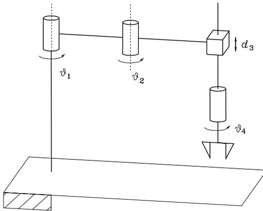
**Fig. 2.36.** SCARA manipulator
