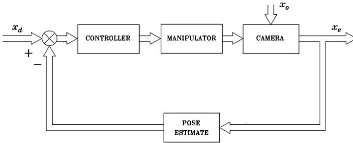
Fig. 10.12. General block scheme of position-based visual servoing
