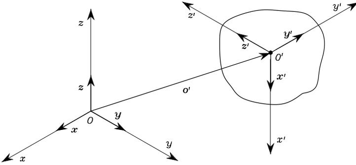
Fig. 2.1. Position and orientation of a rigid body
