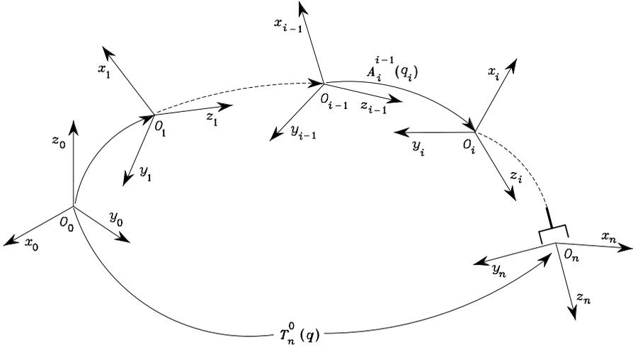
**Fig. 2.15.** Coordinate transformations in an open kinematic chain
