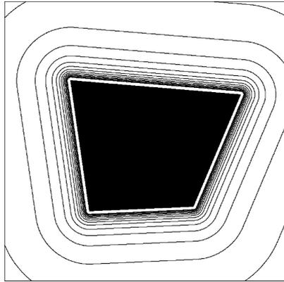
**Fig. 12.13.** The equipotential contours of the repulsive potential  $U_r$  in the range of influence of a polygonal  $\mathcal{C}$ -obstacle in  $\mathcal{C} = \mathbb{R}^2$ , for  $k_r = 1$  and  $\gamma = 2$
