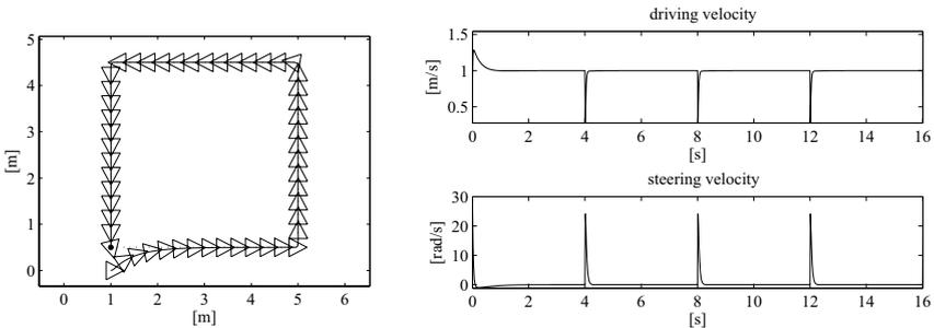
**Fig. 11.17.** Tracking a square reference trajectory (*dotted*) with the controller based on input/output linearization, with  $b = 0.2$ ; *left*: Cartesian motion of the unicycle, *right*: time evolution of the velocity inputs  $v$  and  $\omega$
