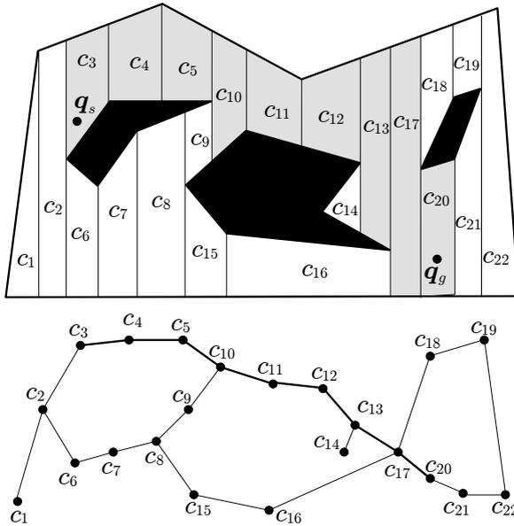
**Fig. 12.7.** An example of trapezoidal decomposition via the sweep line algorithm (above) and the associated connectivity graph (below). Also shown is the solution of a particular planning problem ( $c_s = c_3$  and  $c_g = c_{20}$ ), both as a channel in  $C_{\text{free}}$  and as a path on the graph
