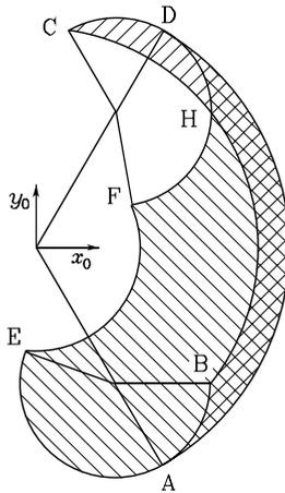
**Fig. 2.30.** Workspace of a two-link planar arm
