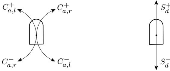
**Fig. 11.11.** The elementary arcs that constitute the trajectories of the sufficient family for the minimum-time planning problem for the unicycle
