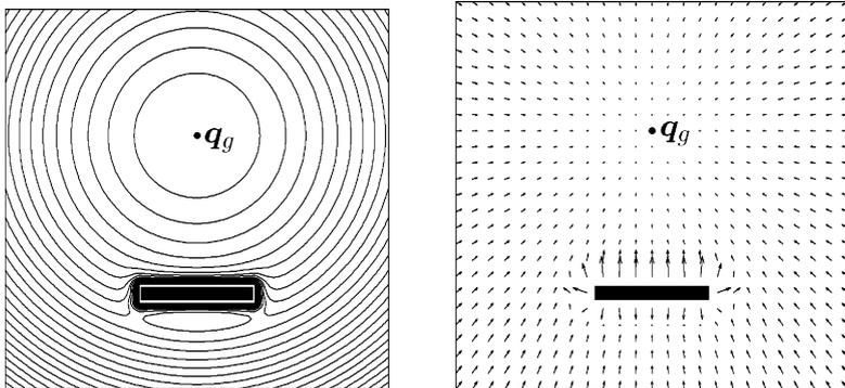
**Fig. 12.14.** The total potential in  $\mathcal{C} = \mathbb{R}^2$  obtained by superposition of a hyperbolic attractive potential and a repulsive potential for a rectangular  $\mathcal{C}$ -obstacle: *left*: the equipotential contours, *right*: the resulting force field
