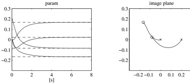
**Fig. 10.21.** Time history of feature parameters and corresponding path of feature points projections on image plane with control **B**
