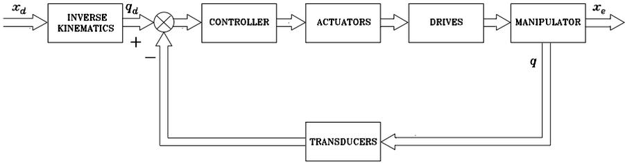
**Fig. 8.1.** General scheme of joint space control
