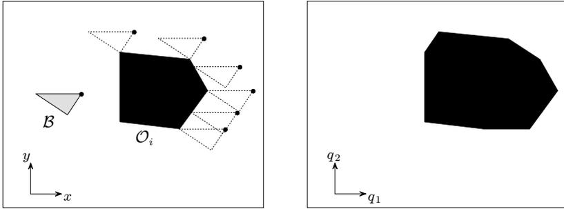
**Fig. 12.3.**  $\mathcal{C}$ -obstacles for a polygonal robot translating in  $\mathbb{R}^2$ ; *left*: the robot  $\mathcal{B}$ , an obstacle  $\mathcal{O}_i$  and the growing procedure for building  $\mathcal{C}$ -obstacles, *right*: the configuration space  $\mathcal{C}$  and the  $\mathcal{C}$ -obstacle  $\mathcal{C}\mathcal{O}_i$
