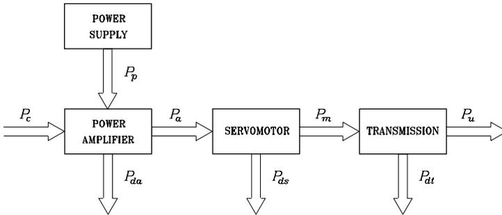
Fig. 5.1. Components of a joint actuating system
