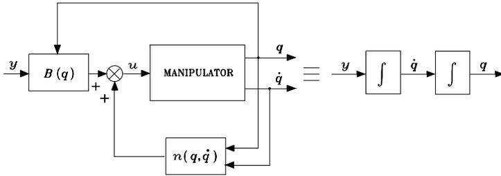
Fig. 8.21. Exact linearization performed by inverse dynamics control
