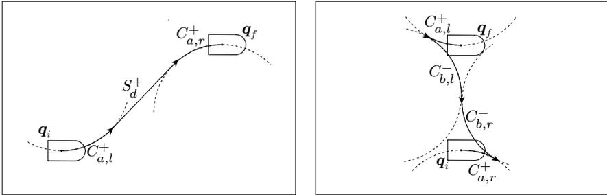
**Fig. 11.12.** Two examples of minimum-time trajectories for the unicycle
