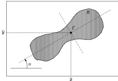
**Fig. 10.4.** Region of a binary image and some feature parameters
