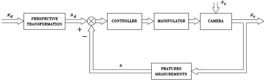
**Fig. 10.13.** General block scheme of image-based visual servoing
