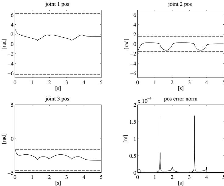
**Fig. 3.20.** Time history of the joint positions and the norm of end-effector position error with the Jacobian pseudo-inverse algorithm and joint limit constraint (joint limits are denoted by *dashed lines*)
