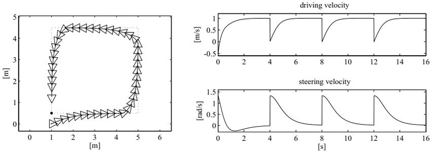
**Fig. 11.16.** Tracking a square reference trajectory (*dotted*) with the controller based on input/output linearization, with  $b = 0.75$ ; *left*: Cartesian motion of the unicycle, *right*: time evolution of the velocity inputs  $v$  and  $\omega$
