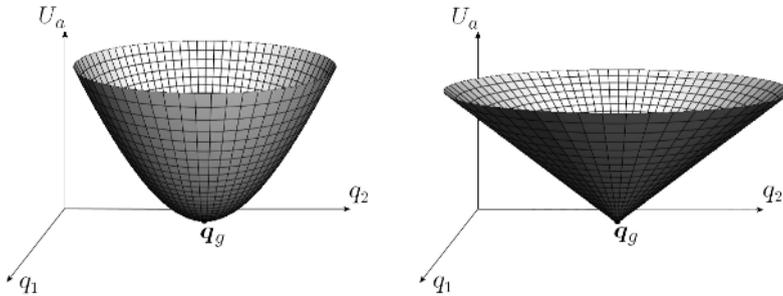
**Fig. 12.12.** The shape of the paraboloidic attractive potential  $U_{a1}$  (left) and of the conical attractive potential  $U_{a2}$  (right) in the case  $\mathcal{C} = \mathbb{R}^2$ , for  $k_a = 1$
