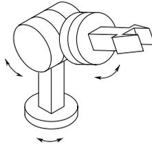
**Fig. 1.11.** Spherical wrist
