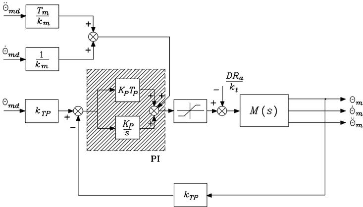
Fig. 8.15. Equivalent control scheme of PI type
