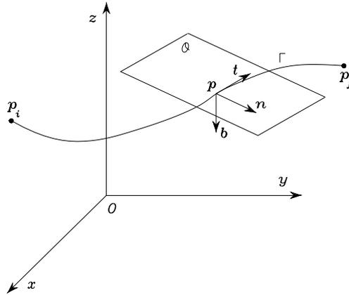
**Fig. 4.11.** Parametric representation of a path in space
