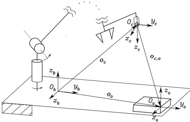
Fig. 10.5. Reference frames for an eye-in-hand camera
