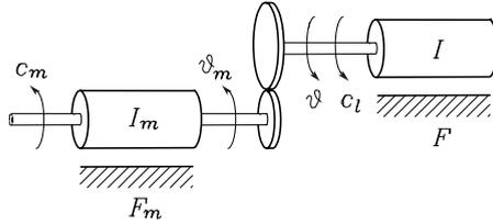
Fig. 5.7. Schematic representation of a mechanical gear
