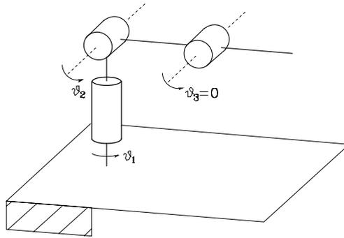
**Fig. 3.5.** Anthropomorphic arm at an elbow singularity
