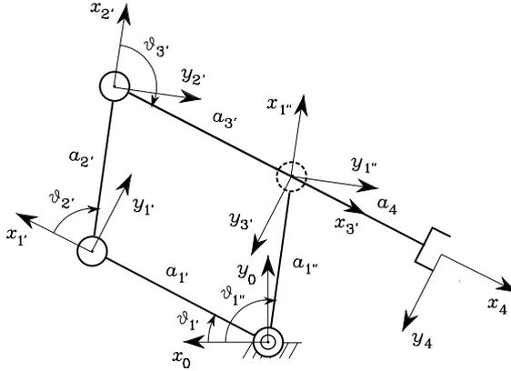
Fig. 2.21. Parallelogram arm
