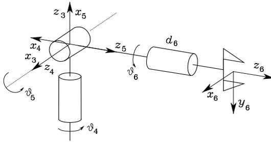
Fig. 2.24. Spherical wrist
