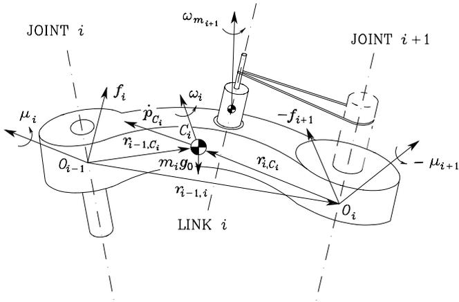
**Fig. 7.13.** Characterization of Link  $i$  for Newton–Euler formulation
