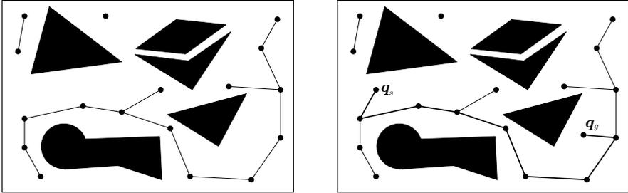
**Fig. 12.9.** A PRM in a two-dimensional configuration space (*left*) and its use for solving a particular planning problem (*right*)
