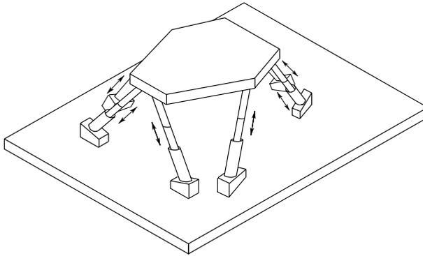
**Fig. 1.9.** Parallel manipulator
