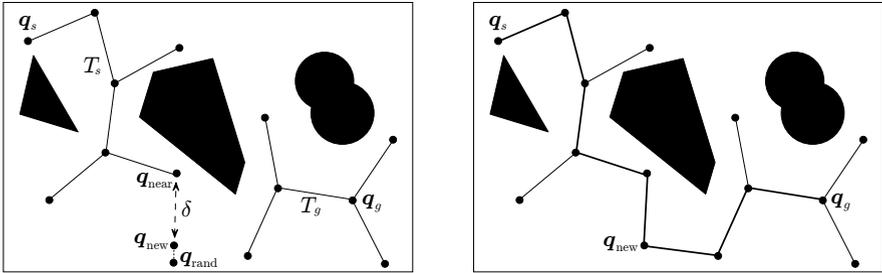
**Fig. 12.10.** The bidirectional RRT method in a two-dimensional configuration space *left*: the randomized mechanism for expanding a tree, *right*: the extension procedure for connecting the two trees
