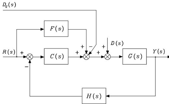
Fig. C.2. Feedback control structure with feedforward compensation
