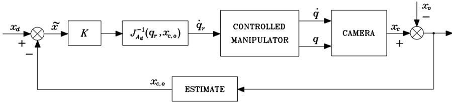
Fig. 10.15. Block scheme of resolved-velocity position-based visual servoing
