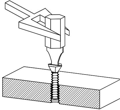
**Fig. 9.17.** Driving a screw in a hole
