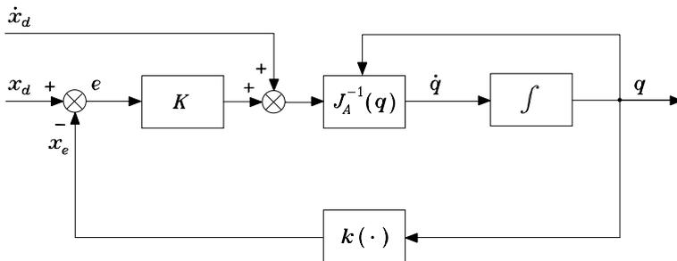
Fig. 3.11. Inverse kinematics algorithm with Jacobian inverse
