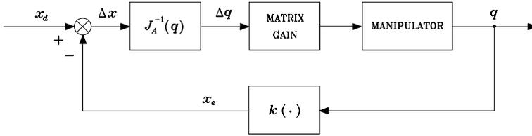
Fig. 8.27. Block scheme of Jacobian inverse control
