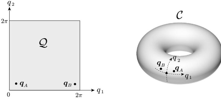
**Fig. 12.1.** The configuration space of a 2R manipulator; *left*: a locally valid representation as a subset of  $\mathbb{R}^2$ , *right*: a topologically correct representation as a two-dimensional torus
