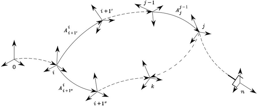
**Fig. 2.18.** Coordinate transformations in a closed kinematic chain
