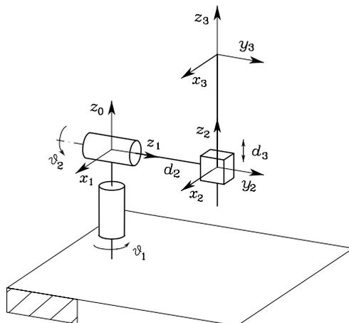
Fig. 2.22. Spherical arm
