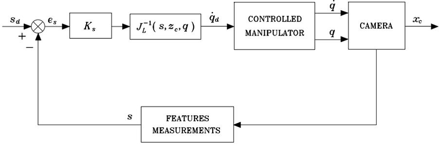
**Fig. 10.17.** Block scheme of resolved-velocity image-based visual servoing
