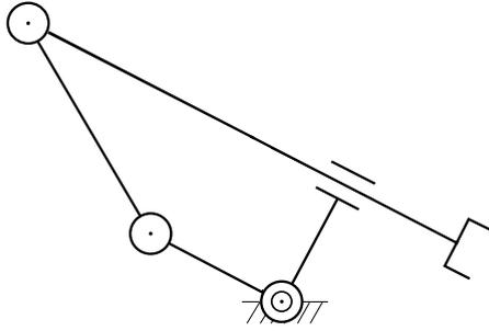
**Fig. 2.34.** Four-link closed-chain planar arm with prismatic joint
