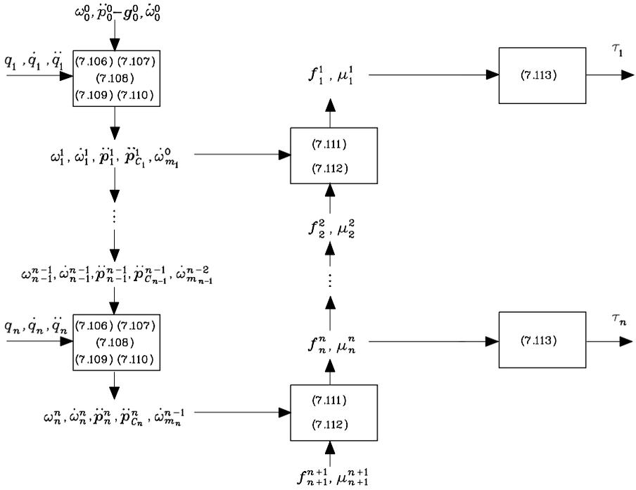
Fig. 7.14. Computational structure of the Newton-Euler recursive algorithm
