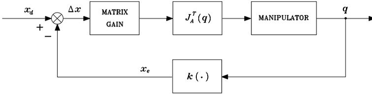
**Fig. 8.28.** Block scheme of Jacobian transpose control
