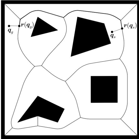
**Fig. 12.5.** An example of generalized Voronoi diagram and the solution of a particular instance of the planning problem, obtained by retracting  $\mathbf{q}_s$  and  $\mathbf{q}_g$  on the diagram. The solution path from  $\mathbf{q}_s$  to  $\mathbf{q}_g$  consists of the two *dashed* segments and the *thick* portion of the diagram joining them
