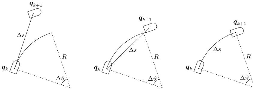
**Fig. 11.21.** Odometric localization for a unicycle moving along an elementary tract corresponding to an arc of circle; *left*: integration via Euler method, *centre*: integration via Runge–Kutta method, *right*: exact integration
