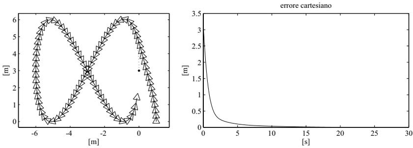
**Fig. 11.15.** Tracking a figure of eight-shaped reference trajectory (*dotted*) with the nonlinear controller; *left*: Cartesian motion of the unicycle, *right*: time evolution of the norm of the Cartesian error  $e_p$
