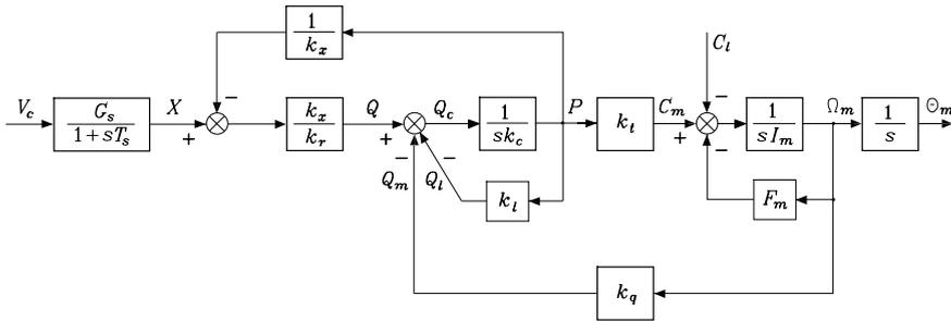
Fig. 5.6. Block scheme of a hydraulic drive
