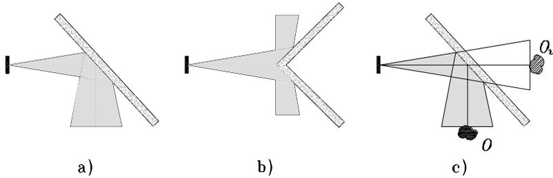
**Fig. 5.19.** Reflector models on smooth surfaces: **a)** non-detected plane. **b)** non-detected corner. **c)** plane with false detection ( $O$  real object,  $O_v$  virtual object detected)
