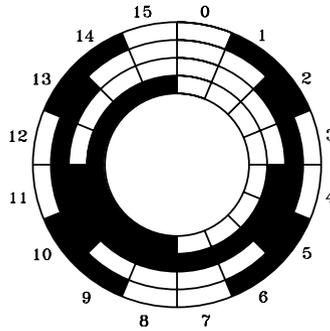
**Fig. 5.12.** Schematic representation of an absolute encoder
