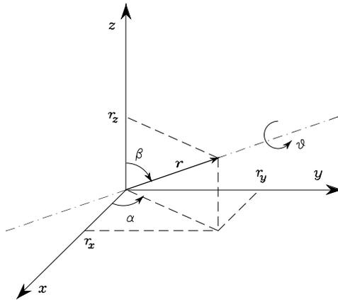
**Fig. 2.10.** Rotation of an angle about an axis
