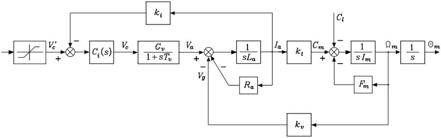
Fig. 5.2. Block scheme of an electric drive
