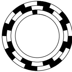
**Fig. 5.13.** Schematic representation of an incremental encoder
