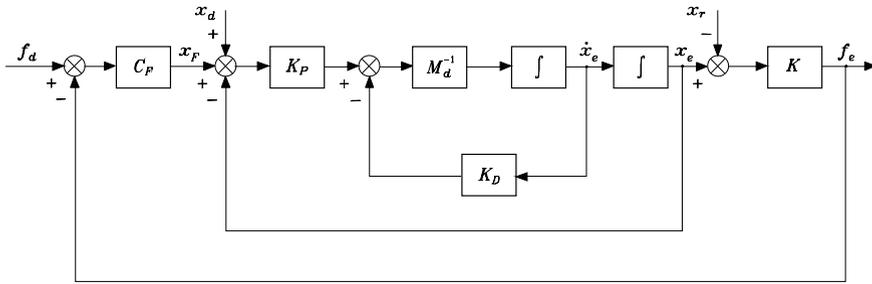
Fig. 9.8. Block scheme of parallel force/position control
