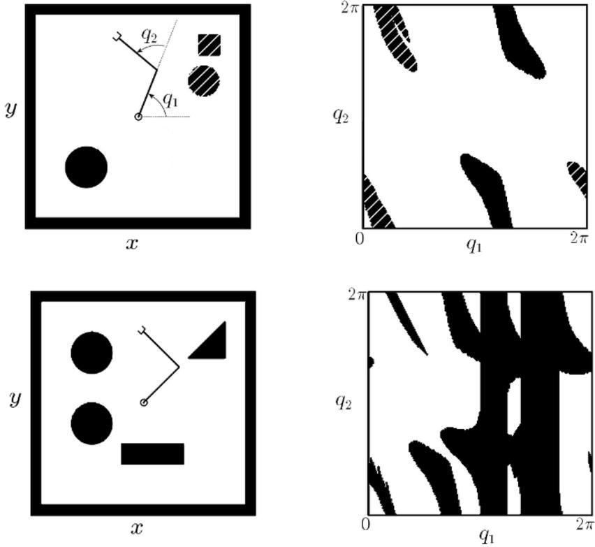
**Fig. 12.4.**  $\mathcal{C}$ -obstacles for a wire-frame 2R manipulator in two different cases; *left*: the robot and the obstacles in  $\mathcal{W} = \mathbb{R}^2$ , *right*: the configuration space  $\mathcal{C}$  and the  $\mathcal{C}$ -obstacle region  $\mathcal{CO}$
