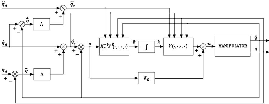
Fig. 8.26. Block scheme of joint space adaptive control
