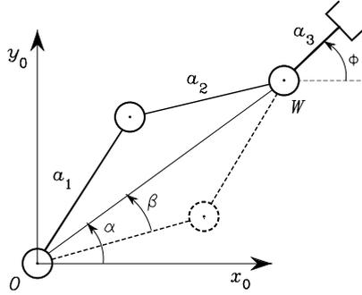
**Fig. 2.31.** Admissible postures for a two-link planar arm
